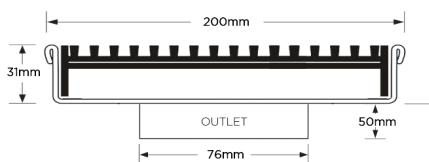
Grates longer than 1500mm supplied in sections. Tile Inserts longer than 1200mm supplied in sections. Channels over 3000mm supplied in sections with joiner. +/-2mm tolerance on dimensions.
