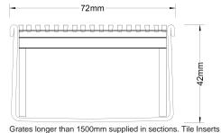
longer than 1300mm supplied in sections. The inserts longer than 1200mm supplied in sections. Channels over 3000mm supplied in sections with joiner. +/-2mm tolerance on dimensions.
