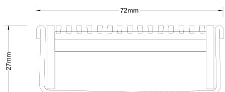
Grates longer than 1500mm supplied in sections. Tile Inserts longer than 1200mm supplied in sections. Channels over 3000mm supplied in sections with joiner. +/-2mm tolerance on dimensions.
